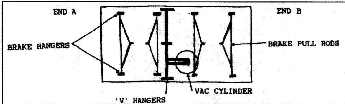
Cut a 44mm length from the fret scrap and solder in place between the solebars, to the right of the V hangers. This is for mounting the vacuum cylinder.
